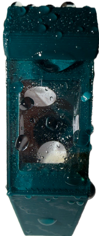
Figure 5.10: Sensor module interior after 50 spray cycles. No color change observed on water-sensitive labels, confirming absence of leakage.
