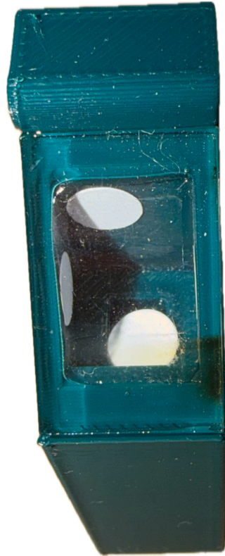
Figure 5.9: Sensor module interior prior to water exposure.
