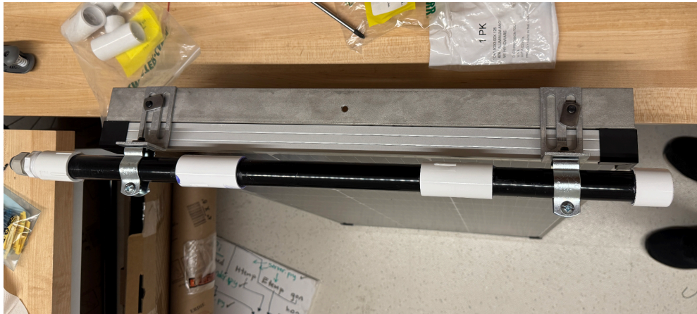
Figure 4.9 The Physical Self-Cleaning Prototype Mounted to the End of the Panel Holder
