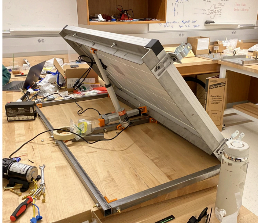
Figure 5.6: Panel rotating successfully about the intended single axis during the testing.
